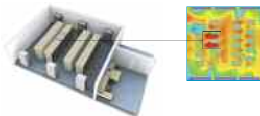
A. Hot spot due to insufficient Cooling
